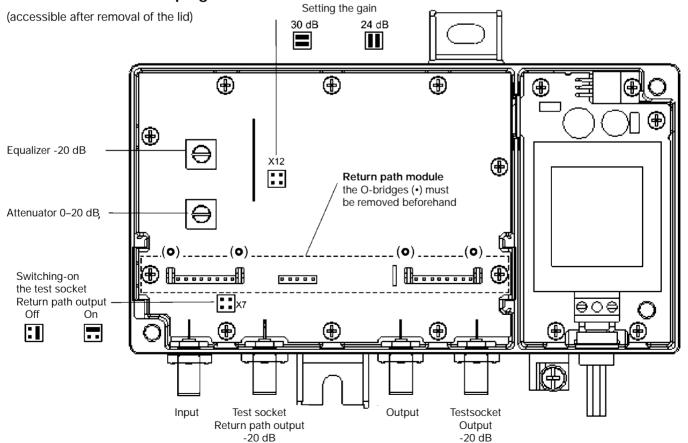
Switching-on with test socket X7. Align the return path. After the measurement: Switch-off with test socket X7.
